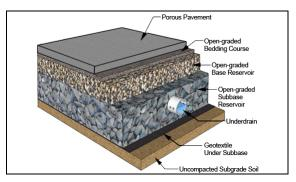
Figure 5-17. Porous Pavement
