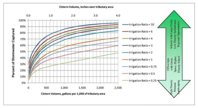
Figure 5-1.Rainwater Harvesting Systems Performance (Geosyntec, 2009)
