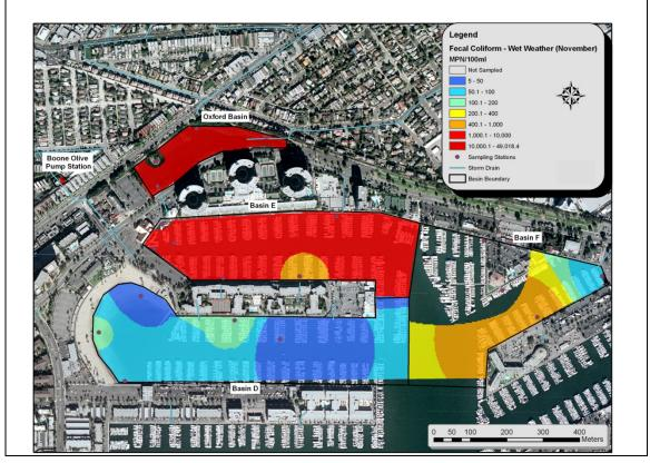
Figure 3-2. Wet Weather Interpolation for Fecal Coliforms (WESTON, 2007)
